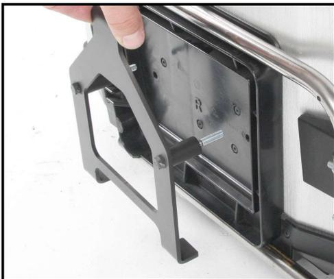
Fit the sealing washers  $\varnothing 6,4 \times \varnothing 16$  on the threads of the locking device. Hang the case into the carrier. Insert the locking device from the outside into the drilled holes.
